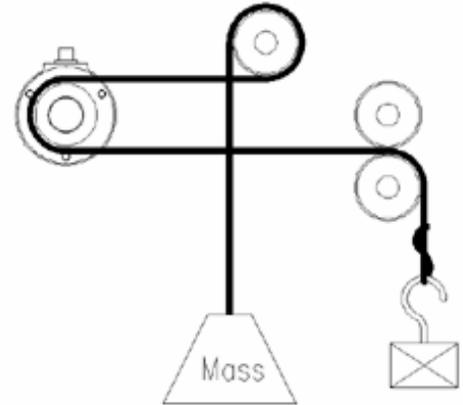
In this example, by rearranging the anchor point and the force location as well as utilizing the idle roll, the frictional losses are minimized.
