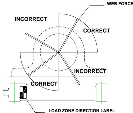
Figure 11 Transducer load direction Diagram.
