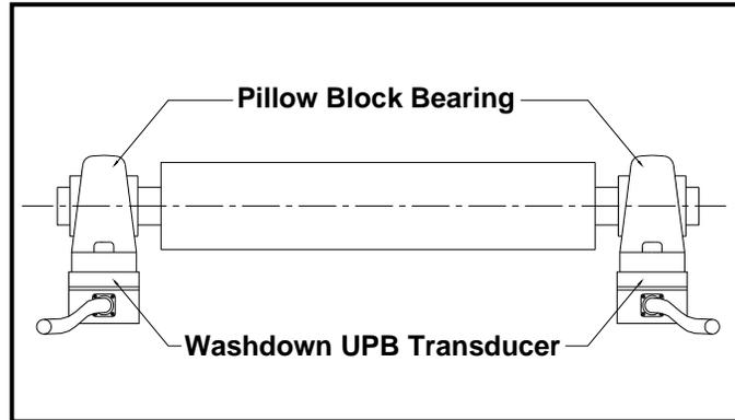
Figure 6 Dual UPB Transducer Application
