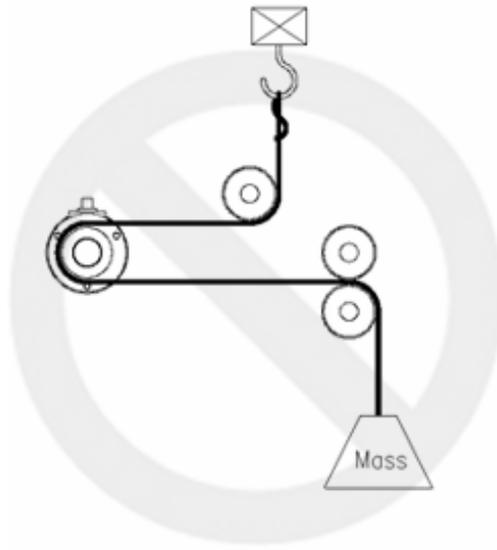
In this example, only a fraction of the test force is transferred to the transducer due to drag from the driven roll.
