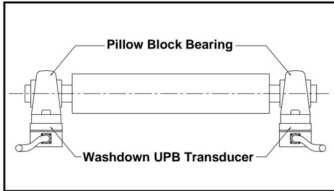
**Figure 9 Mounting Configuration**
