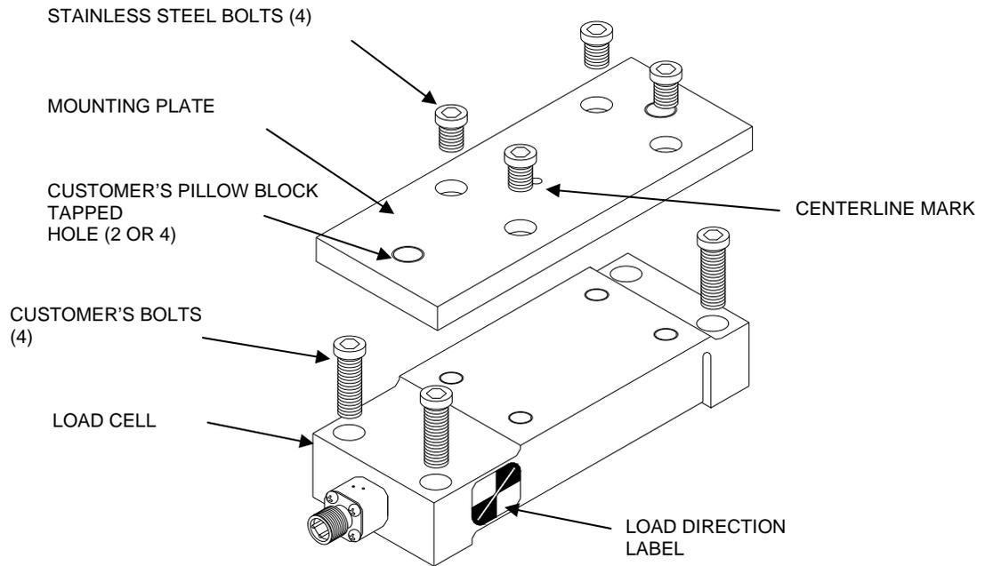
Figure 12 Mounting the Under Pillow Block Transducer
