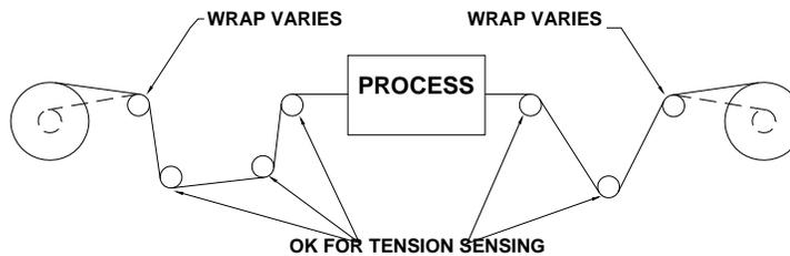
**Figure 10 Example of Varying Wrap Angles**
