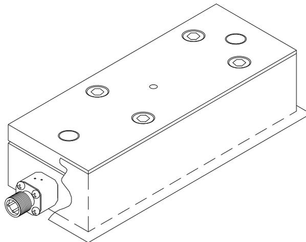
Figure 13 Mounting the Under Pillow Block Transducer
