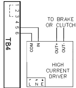
High Current Driver connections for 0-10V input
