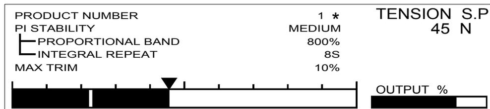
Access the Adjust PI stability menu from the Commissioning menu. Run the machine with the Controller in Auto at a Tension Set Point of approximately 50%. Use the SCROLL keys to select the parameter to be changed and adjust the parameter using the numeric keys or the +/- keys. Press the CONFIRM key to implement and save the change. An asterisk alongside the Product Number indicates that a parameter has been changed and that the CONFIRM key must be pressed to implement and save the change.
