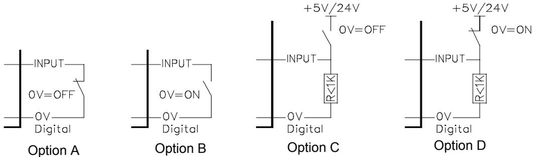
The digital input is shown in the OFF position
