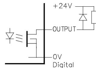
When mains powered, the total current that can be taken from the Controller 24V DC supply by the digital outputs is 50mA maximum. When 24V DC powered this current will depend on the users supply.
