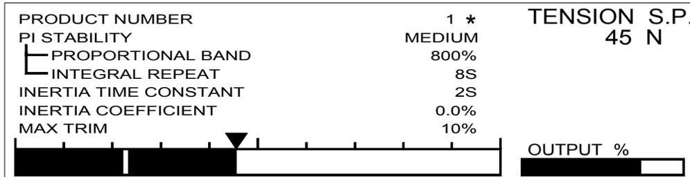
Access the Adjust PI stability menu from the Commissioning menu. Run the machine with the Controller in Auto at a Tension Set Point of approximately 50%. Use the SCROLL keys to select the parameter to be changed and adjust the parameter using the numeric keys or the +/- keys. Press the CONFIRM key to implement and save the change. An asterisk alongside the Product Number indicates that a parameter has been changed and that the CONFIRM key must be pressed to implement and save the change.
