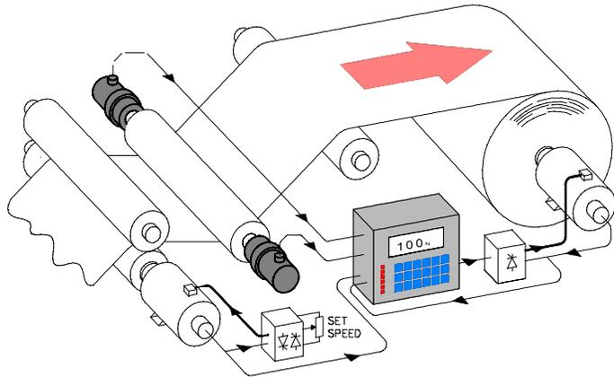
A motor driven center winder with taper feature
