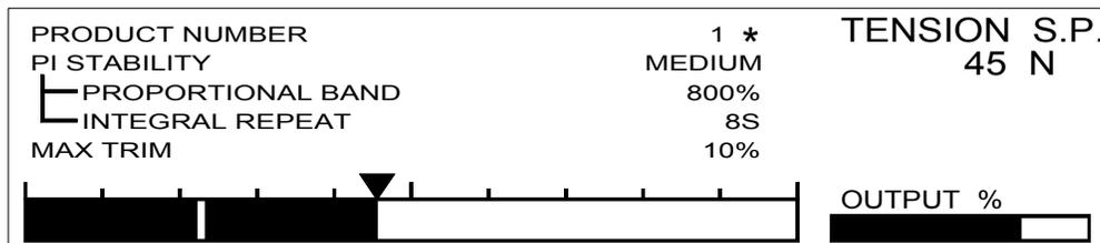
Access the Adjust PI stability menu from the Commissioning menu. Run the machine with the Controller in Auto at a Tension Set Point of approximately 50%. Use the SCROLL keys to select the parameter to be
