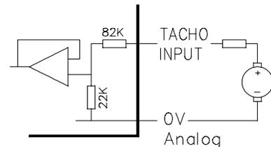
**Under/over winding;** the polarity of the line and winder tachos must be switched externally to provide positive tacho inputs to the Controller.
