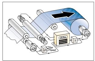
A center winder with taper tension
