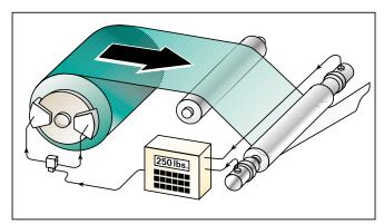
An unwind system with dual range disc brake
