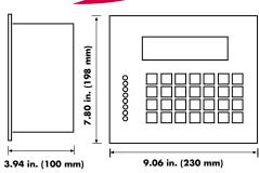
Standard Mounting Cut-Out 8.27 in. (210 mm) X 7.01 in. (178 mm)
