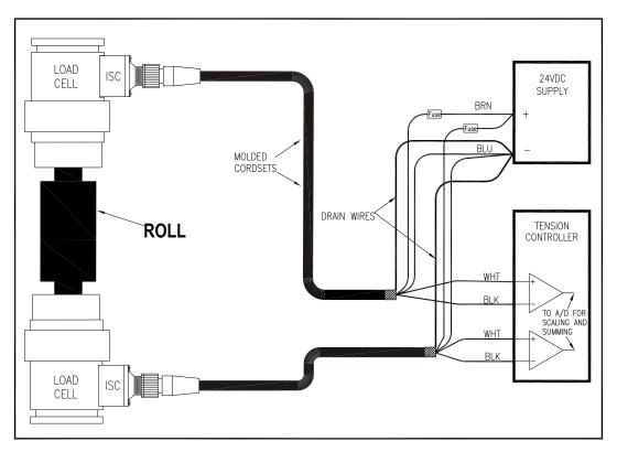
**Figure 5 Installation Wiring Diagram**
