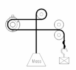
In this example, only a fraction of the test force is transferred to the transducer due to drag from the driven roll. In this example, by rearranging the anchor point and the force location as well as utilizing the idle roll, the frictional losses are minimized.
