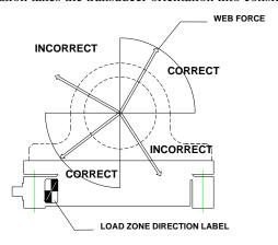
Figure 11 Transducer load direction Diagram.
