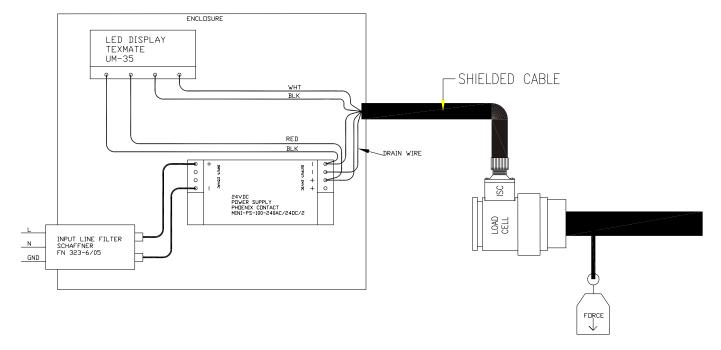
Figure 14 EMC Connections and Installation
