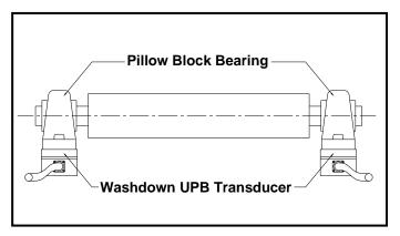
**Figure 9 Mounting Configuration**
