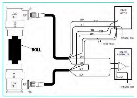
Figure 8 Stacking the Two Loadcell Outputs
