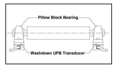
Figure 6 Dual UPB Transducer Application
