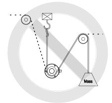
In this example, the true web path was difficult to access and an incorrect path was implemented using a convenient, but incorrect anchor point.
