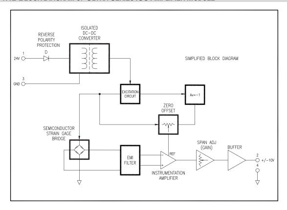
Figure 2 Block Diagram of Ultra Series ISC Amplifier Module
