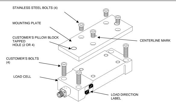
Figure 12 Mounting the Under Pillow Block Transducer
