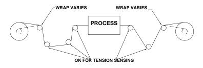
Figure 10 Example of Varying Wrap Angles
