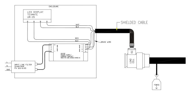
Figure 12 EMC Connections and Installation
