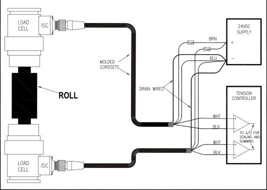
Figure 5 Installation Wiring Diagram
