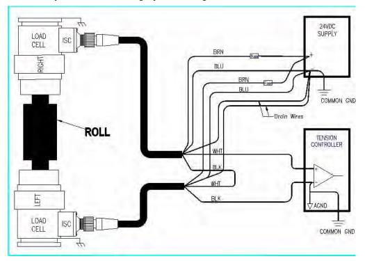
Figure 8 Stacking the Two Loadcell Outputs
