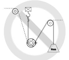
In this example, there was a disregard for maintaining the correct wrap angle. The dotted line indicates the proper web path.
