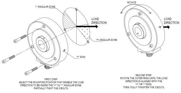
Figure 11 – Positioning the Slim Cell Transducers for Mounting
