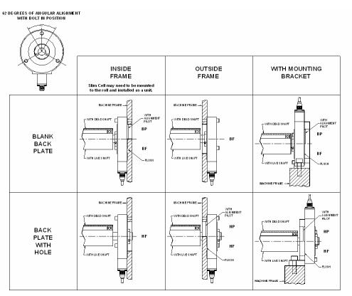
Figure 10- Slim Cell Transducer Mounting Styles
