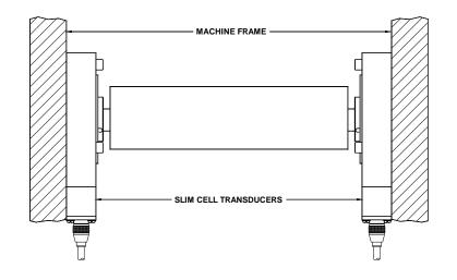
Figure 6- Slim Cell Transducer Incorporating Shaft Bearing Function
