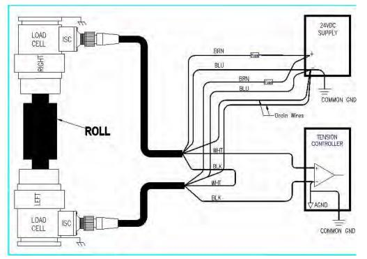
Figure 9 Stacking the Two Loadcell Outputs
