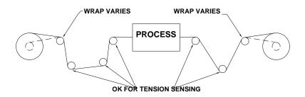
Figure 11 - Example of Varying Wrap Angles
