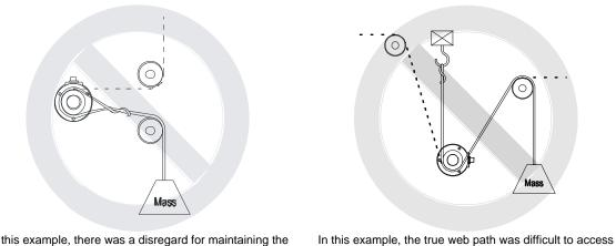
In this example, there was a disregard for maintaining the correct wrap angle. The dotted line indicates the proper web path.
