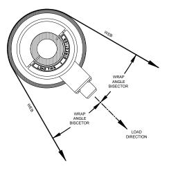
Figure 13 - Proper Orientation of the Cartridge Transducer
