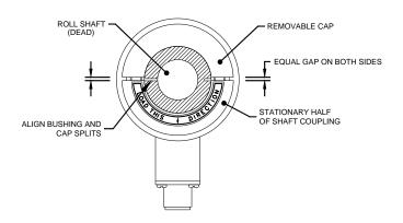
Figure 14 - Correct Shaft Coupling Installation
