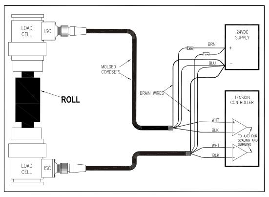
Figure 6 Installation Wiring Diagram
