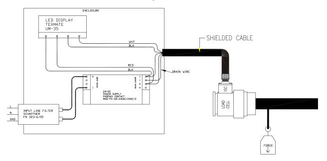
Figure 15 EMC Connections and Installation
