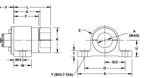
TYPE EC AND ECM CARTRIDGE WITH PB MOUNTING KIT
