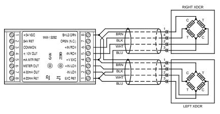
Figure 7 – Full Bridge Transducer Wiring
