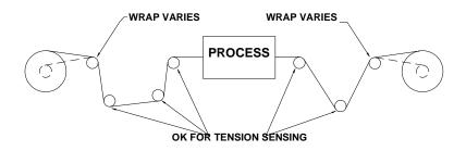
Figure 2 - Example of Varying Wrap Angles
