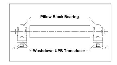
Figure 1 – Mounting Configuration
