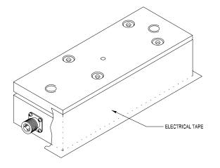
Figure 6 – Mounting the Under Pillow Block Transducer
