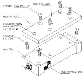
Figure 5 – Mounting the Under Pillow Block Transducer
