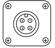
Figure 8 - Front View of M12 Connector
