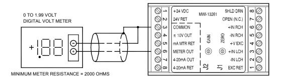
Figure 11 - Output Wiring, Damped +/- 2V Analog
