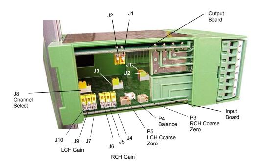
Figure 4 - Internal Jumper-switches and Potentiometer Location
