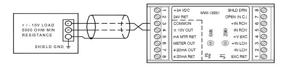
Figure 7 - Output Wiring, +/- 10V Analog
