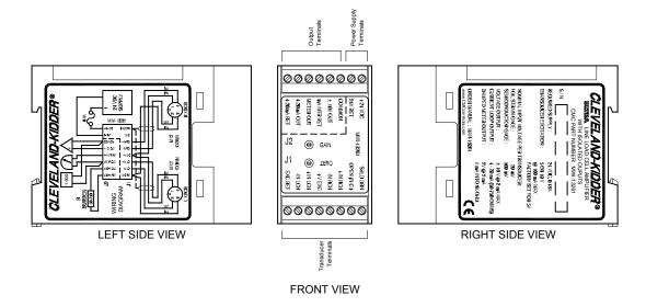
Figure 2- Front and Side Views of Ultra Series DIN Rail Amplifier MWI -13261
