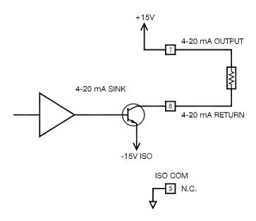
Figure 9 - 4-20 mA Output Circuit Wired for Floating Burden
