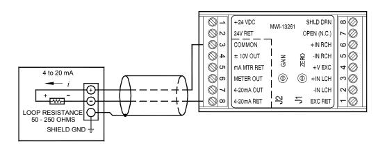
Figure 10 - 4-20 mA Output Wiring for Ground Referred Burden
