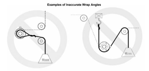
In this example, there was a disregard for maintaining the correct wrap angle. The dotted line indicates the proper web path.
