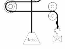
In this example, only a fraction of the test force is transferred to the transducer due to drag from the driven roll.
