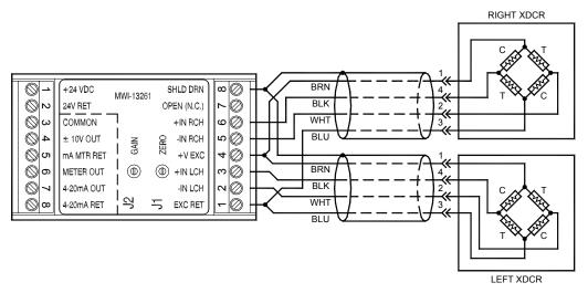
Figure 5 - Full-bridge Transducer Wiring
