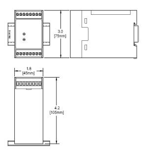
Figure 3 - Ultra Series DIN Rail Amplifier Mounting Diagram
