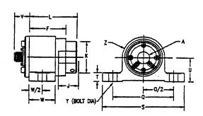
Type CLTEC Cartridge with Pillow Block Mounting Kit
