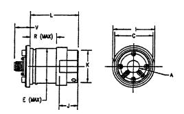
Type CLTEC Cartridge with BR Mounting Kit
