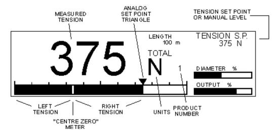
The maximum rate of change of the manual output is determined by the "Set point ramp rate" value. The Set Taper key does not operate. The Manual feature is only available in Unwind Brake mode. The Auto Tension set point may be set with the numeric keys followed by ENTER or by the +/- keys. The analog tension set point triangle is only visible when the Controller is in Auto control. The measured tension analog bar graph and the set point triangle should coincide when in control.
