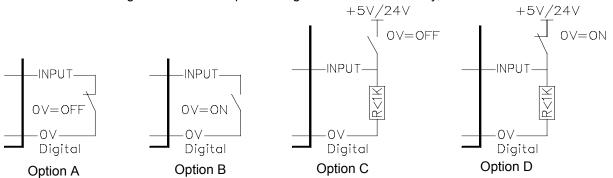
The digital input is shown in the OFF position
