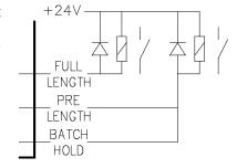
As shown alongside, the output will be held at the Pre Length and will be released when the RESET LENGTH key is pressed.
