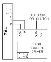
High Current Driver connections for 0-10V input
