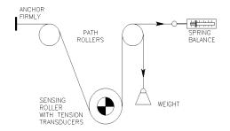
After calibrating the tension, return to the Control screen and verify that the display shows zero when no tension is being measured and that the display shows the correct tension value when the weight or spring balance force is applied.
