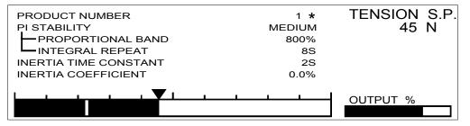
Access the Adjust PI stability menu from the Commissioning menu. Run the machine with the Controller in Auto at a Tension Set Point of approximately 50%. Use the SCROLL keys to select the parameter to be changed and adjust the parameter using the numeric keys or the +/- keys. Press the CONFIRM key to implement and save the change. An asterisk alongside the Product Number indicates that a parameter has been changed and that the CONFIRM key must be pressed to implement and save the change.
