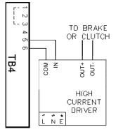
High Current Driver connections for 0-10V input
