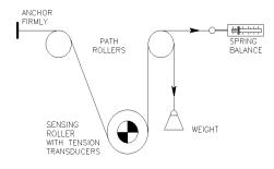
The Controller will calibrate both transducers simultaneously. The rope must be in the exact center of the web path so that each transducer is equally loaded.
