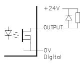
When mains powered, the total current that can be taken from the Controller 24V DC supply by the digital outputs is 50mA maximum. When 24V DC powered this current will depend on the users supply.
