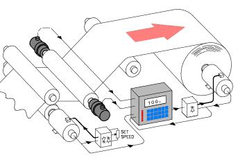
A motor driven center winder with taper feature
