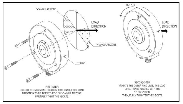
output signal of the transducer is positive. If the force points to the "-" the output is negative. This is importance to know when wiring the transducer to the amplifier, indicator, or controller terminals. Interchanging the B (black wire) and C (red wire) connections may be required in order to provide the proper signal polarity for the device. (see **Figure 6**).
